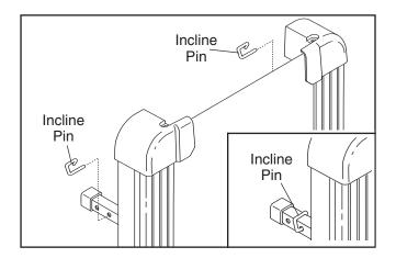
Adjust the other incline leg in the same way. Make sure that both incline pins are inserted from the direction shown in the drawing.
